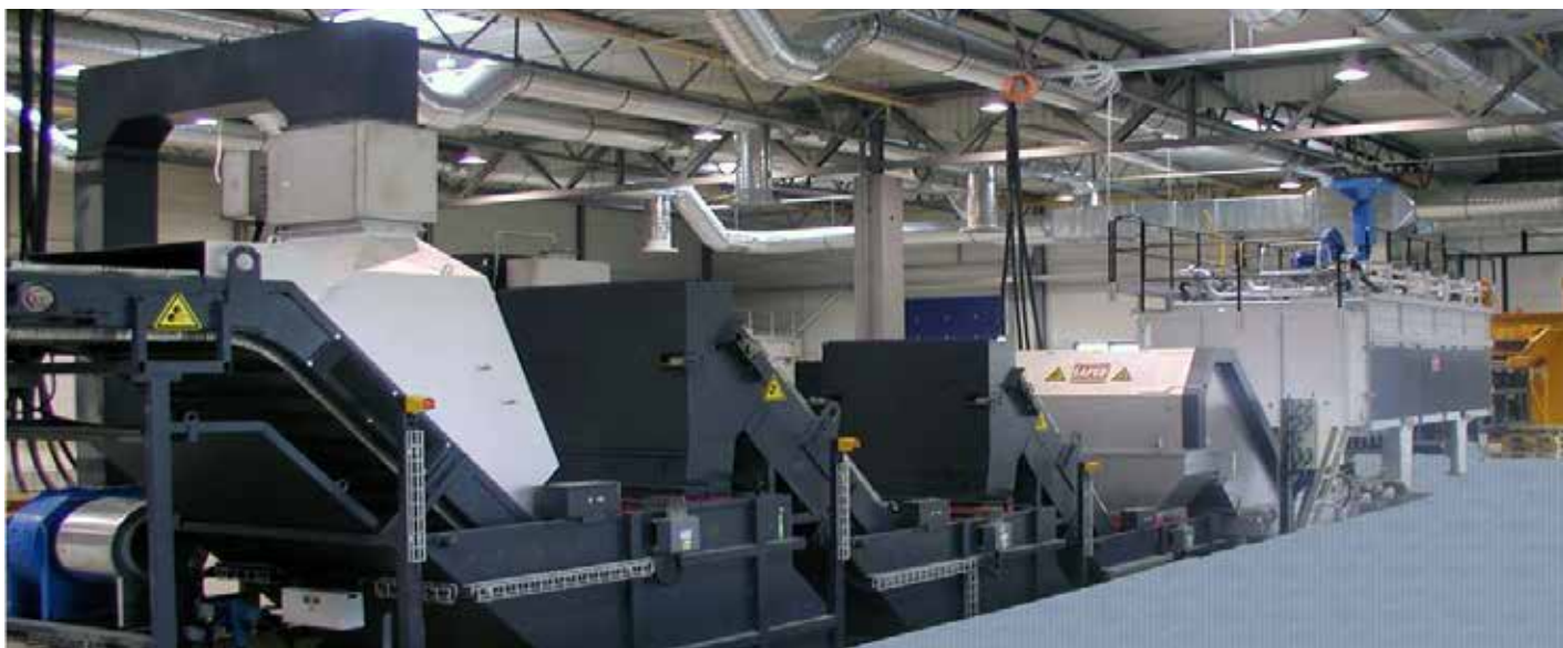
Type T plant 80/54 for carbonitriding screws; throughput rate approx. 370 kg/h; gas-heated.
